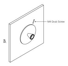
Fit the circular wall plate over the mounting plate and secure with the supplied M4 grub screw at the top of the plate.
