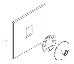
Unscrew the grub screw to seperate the screw plate from the circular face plate.
