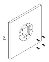
Install the screw plate to the wall using appropriate fasteners for the wall substrate.
