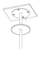
Secure the magnetic cover plate onto the mounting plate.
