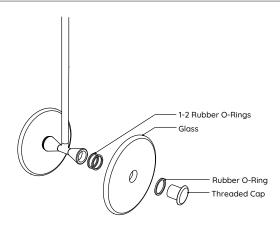
To install the glass piece, hold the glass against the LED housing and thread the 30mm threaded cap into the LED housing.
