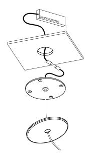
Prep the ceiling with an approx. 40-60mm hole. Connect the single electrified cable to the transformer and place it into the ceiling cavity.
