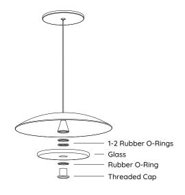
To install the glass piece, hold the glass against the LED housing and thread the 30mm threaded cap into the LED housing.
