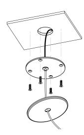
Screw the mounting plate to the ceiling using appropriate fasteners for the ceiling substrate.
