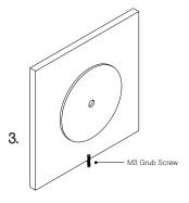
Prep the wall with an approx. 5-20mm hole. Secure the transformer into the wall cavity and feed the cable through the hole into the room. Connect the single electrified cable to the transformer.
