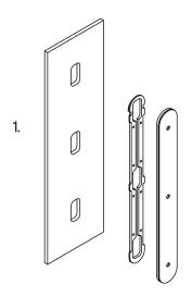
Prep the wall with 3 holes to match the wall plate cutouts. Secure the transformer into the wall cavity and feed the cable through the hole into the room. Connect the single electrified cable to the transformer.
