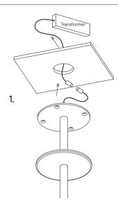
Prep the ceiling with an approx. 5–15mm hole. Place the transformer in the ceiling and feed the cable through the hole into the room. Connect the single electrified cable to the transformer.
