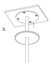
Secure the magnetic cover plate onto the mounting plate.
