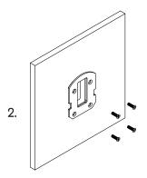
Install the screw plate to the wall using appropriate fasteners for the wall substrate.
