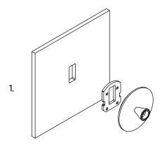
Unscrew the grub screw to seperate the screw plate from the circular face plate.
