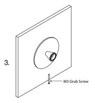
Fit the circular wall plate over the mounting plate and secure with the supplied M3 grub screw at the bottom of the plate.
