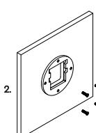
Install the screw plate to the wall using appropriate fasteners for the wall substrate.
