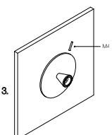
Fit the circular wall plate over the screw plate and secure with the supplied M4 screw at the top of the plate.
