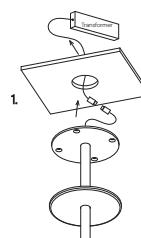
Prep the ceiling with an approx. 50mm hole to fit the transformer. Place the mounting plate in the ceiling and feed the cable through the hole into the room. Connect the single electrified cable to the transformer.
