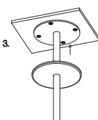
Secure the magnetic cover plate onto the mounting plate.
