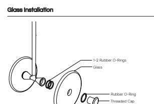
To install the glass piece, hold the glass against the LED housing and thread the 50mm threaded cap into the LED housing.
