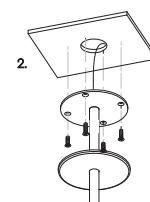
Screw the steel mounting plate to the ceiling using appropriate fasteners for the ceiling substrate.
