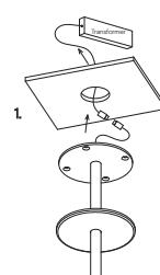
Prep the ceiling with an approx. 50mm hole to fit the transformer. Place the transformer in the ceiling and feed the cable through the hole into the room. Connect the single electrified cable to the transformer.
