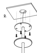
Screw the steel mounting plate to the ceiling using appropriate fasteners for the ceiling substrate.
