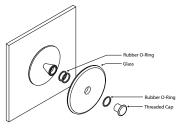
To install the glass piece, hold the glass against the LED housing and thread the 30mm threaded cap into the LED housing. \*Ensure the rubber o-rings are installed in the correct position, 1 behind the glass, and 1 in-front on the glass. If the glass is not held firmly when the threaded cap is fully screwed in, install an extra o-ring.
