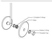
To install the glass piece, hold the glass against the LED housing and thread the 30mm threaded cap into the LED housing.
