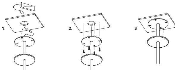
Prep the ceiling with an approx. 50mm hole to fit the transformer. Place the transformer in the ceiling and feed the cable through the hole into the room. Connect the single electrified cable to the transformer.
