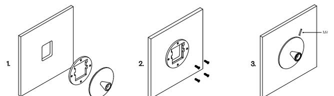
1. Unscrew the grub screw to separate the screw plate from the circular face plate.
