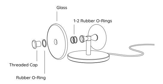
To install the two glass pieces, hold the glass against the LED housing and thread the 30mm threaded cap into the LED housing.
